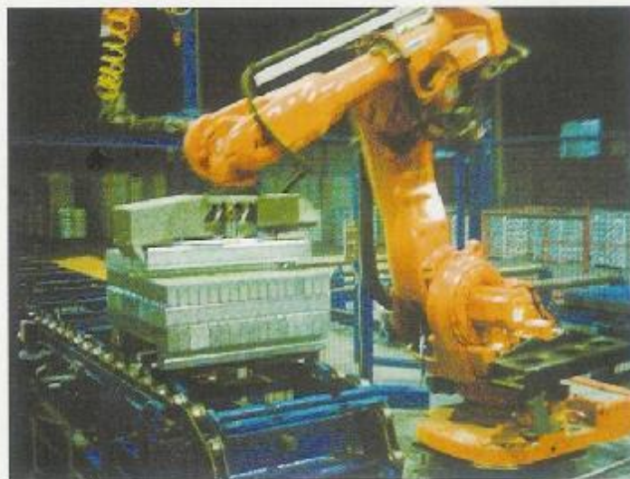
Fig. 5: Robotic stacking device
