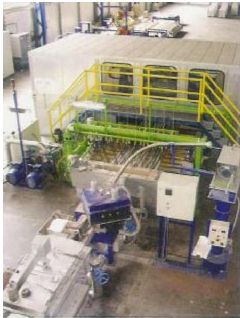
Fig. 1: Gautschi horizontal DC casting machine
