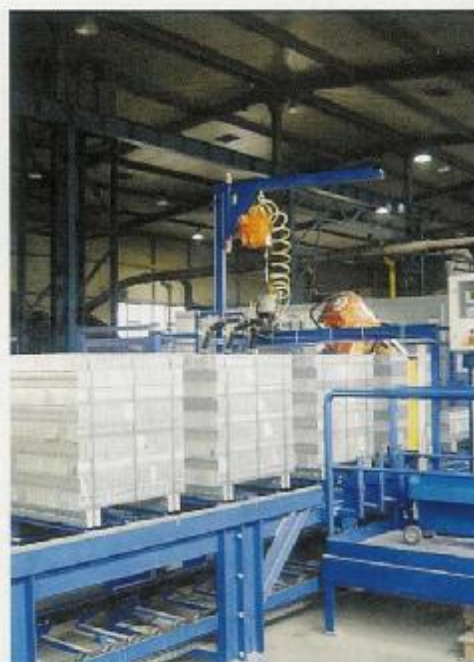
Fig. 6: Semi-automatic strapping system
